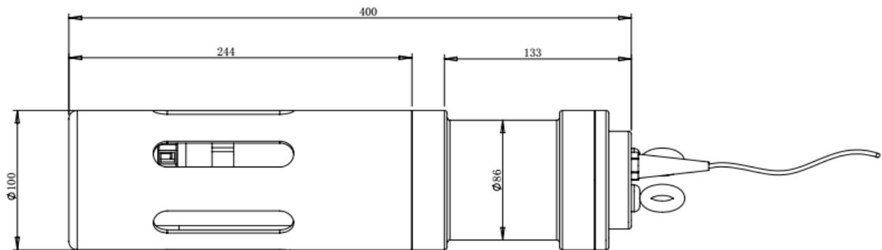
Note: Use lifting rings or pipe threads to install the sensor to avoid direct stress on the cable. The sensor connector is M16-5 cores male waterproof connector.
